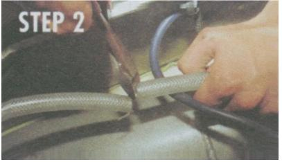
**Step 2:** When you cut the hose for the flow control valve installation, shorten it approximately one and a half to two inches (This is the length of the Jetworks flow control valve).
