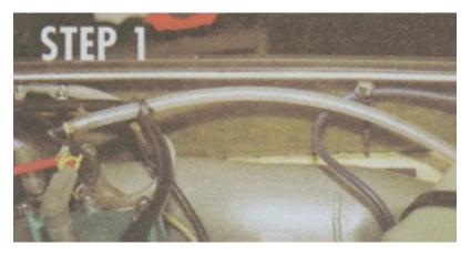
**Step 1:** You have got the standard hose going from the headpipe to the stinger. Take note that most of the engine's cooling water is run through this hose after cooling the engine and headpipe.
