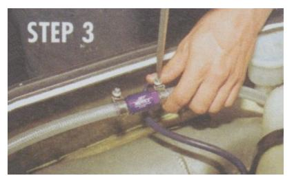
**Step 3:** Place the flow control valve between the hose ends with the arrow pointing toward the stinger. Tighten clamps. The valve is externally adjustable; you can turn the latter by hand without loosening the clamps.
